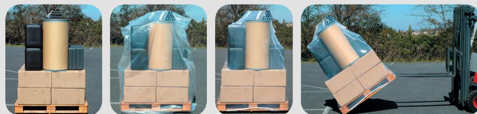
The film takes on the shape of the product by shrinking under the heat produced by the RIPACK® SERIES 3000. The film forms an excellent protective layer and thermal barrier. The objects are held together and the heat transferred is minimal.
