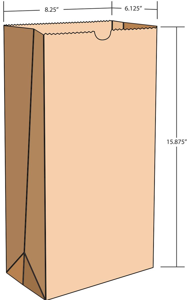
A gusset is a triangle shaped fold on either side of a bag. The gusset is considered the depth of a bag.
