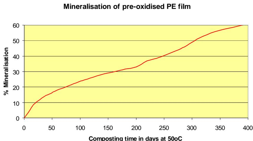
It can be seen that after approximately 400 days of laboratory composting at 50oC, 60% of the available Carbon had been mineralised.
