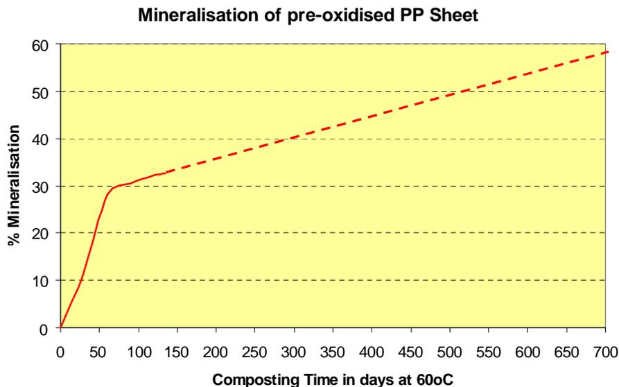
This experiment was terminated after 135 days when a value of approximately 33% was achieved. However, extrapolation of the data strongly indicates that 60% mineralisation will occur after approximately 700 days of composting.
